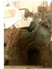
Figure 2: Arching and ratholing on site
