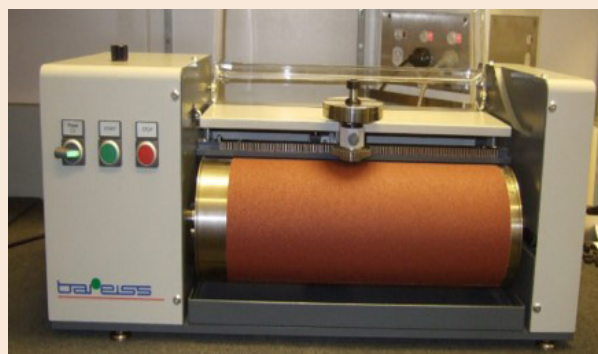
Figure 3: Abrasion Resistance Standard of Cover Rubber
