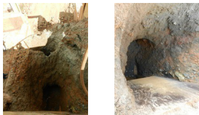
Figure 2: Arching and Ratholing on Site
