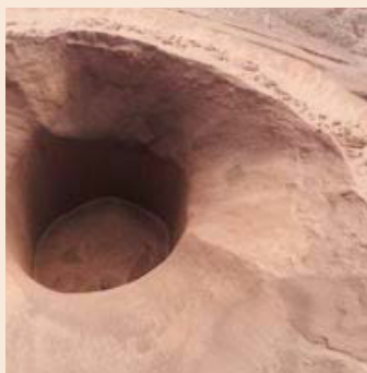
Figure 2: Rathole Formation Reducing Live Capacity
