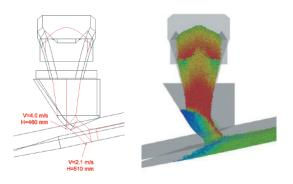
**Continuum** – granular dynamics based on bulk density and friction – predicts velocities and burden depths
