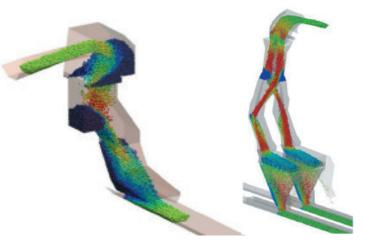
**DEM** – parameters are selected based on calibration testing – excellent visualisation tool as well as allowing numerical analysis
