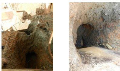
Figure 2: Arching and Ratholing on Site
