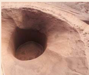
Figure 2: Rathole Formation Reducing Live Capacity
