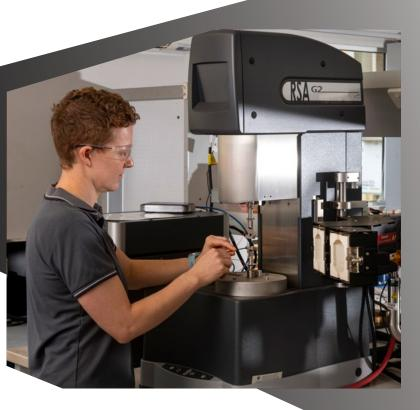
TUNRA Bulk Solids can carry out large scale indentation rolling resistance testing according to AS 1334.13, which is referenced in CEMA 7<sup>th</sup> Edition.
