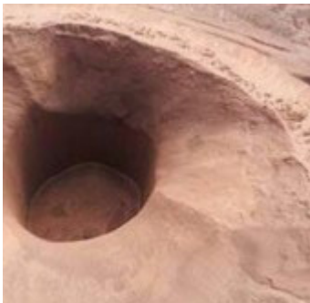
Upgrade of Iron Ore Gravity Reclaim Stockpile to increase Live Capacity. a) Rathole formation reducing live capacity; b) Post-modifications stockpile drawdown
